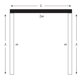
The two rods on the arms of the U each have mass m; the third rod has mass 2m. How far below the midpoint of the horizontal rod is the center of mass of this assembly?
